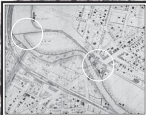
ON THIS 1870 MAP, THE MILLRACE RUNS FROM ABOVE THE DAM, CIRCLED LEFT, TO POWER THE WOOLLEN MILL, FLOUR MILL, AND THE AGRICULTURAL WORKS, CIRCLED RIGHT.
