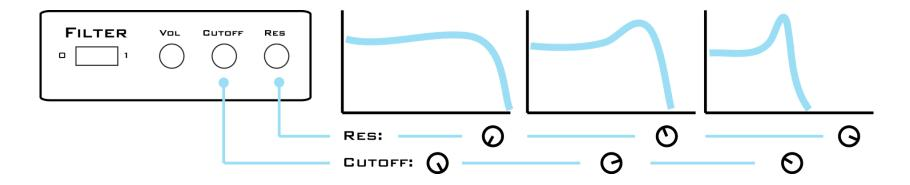
THE NTH'S FILTER IS VERY AGGRESSIVE. HIGH RESONANCE LEVELS CAN RESULT IN DISTORTED, RAW, AND NOISY SOUNDS. FOR A SWEETER TONE, ROLL THE RESONANCE KNOB COUNTER-CLOCKWISE.
