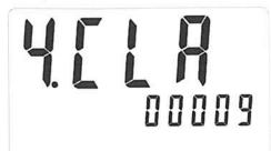
Press "REC" key to clear data logger memory for last record and exit the mode.
