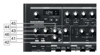
The Arpeggiator is enabled by pressing the On button  $\boxed{42}$ ; the associated LED will confirm its status.
