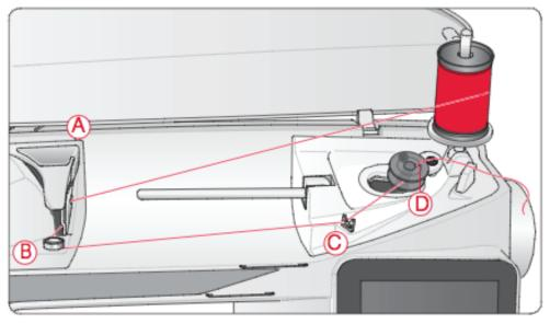
5. Push the bobbin spindle to the right. Hold the end of the thread firmly, and press the foot control to start winding. When the bobbin is full, it will stop rotating. Push the bobbin spindle back to the left, remove the bobbin, and cut the thread.
