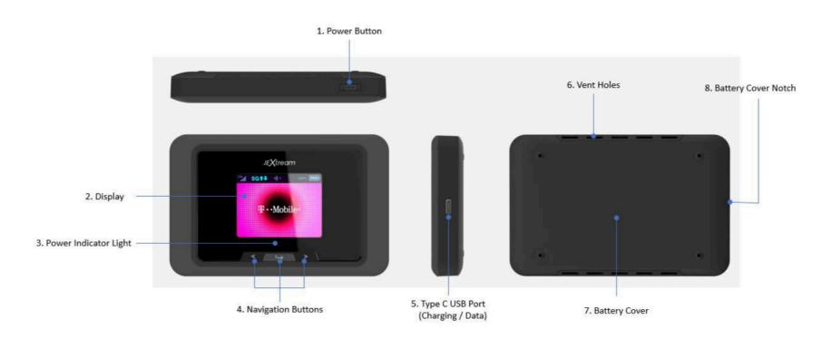
1. Power Button - Turn on/off the device.
