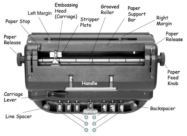
Arrows on paper feeder knobs indicate direction for turning to locked position and for rolling paper out.
