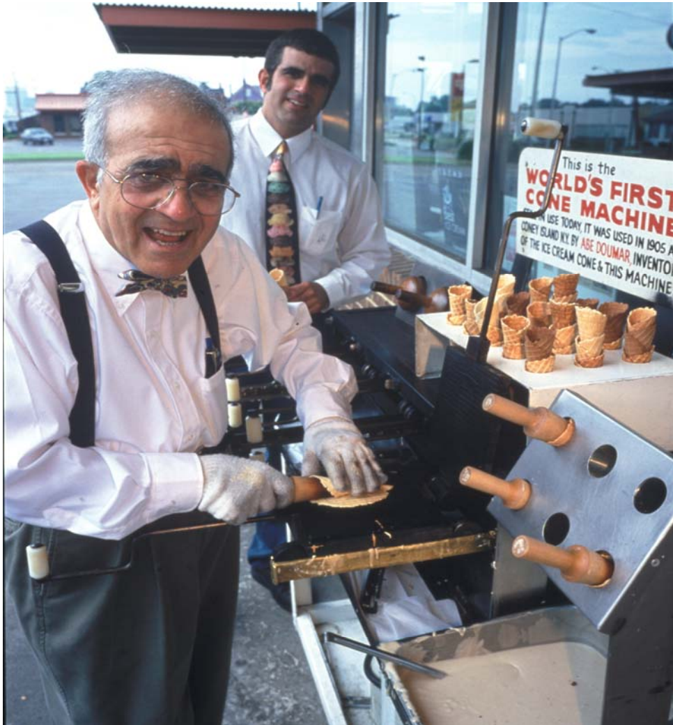
Albert Doumar, owner of Doumar's Cones and Barbecue in Norfolk, VA, shows how to turn wafer-style zalābiyya into an ice-cream cone. The disk-shaped pastry is cooked like a waffle between metal plates, then rolled around a wooden mold while still warm and pliable. It soon cools to a crisp. Doumar's uncle, Abe Doumar, was one of several Syrian-American vendors who recalled fashioning ice-cream cones in this way as an innovation at the 1904 world's fair in St. Louis.
