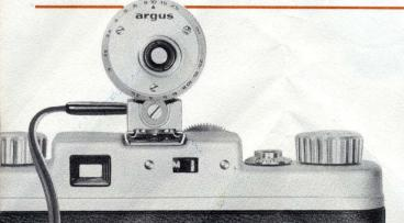
Special outlets on the side of the viewfinder allow the use of flash with the Argus C44 and Argus Flash Extension Bracket. Mount the Flash Extension Bracket on your C44 with the case safety screw, then plug the cord into the viewfinder's outlets. Mount the C44 Flash Unit on the Flash Extension Bracket as you would on the camera.
