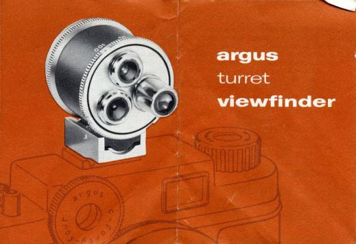
Your Argus Turret Viewfinder features a precision, selective optical system to show exactly what you are photographing with the 35mm Wide Angle, 50mm Normal, or 100mm Telephoto Lens. Your view will always be magnified to the full proportions of the viewfinder, not reduced in size. An efficient adjustment compensates for parallax—the difference which would otherwise occur between the views covered by the lens and the viewfinder. You see precisely what the lens sees—at all distances.
