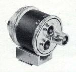
With the viewfinder in place on the camera, set the turret on the front of the finder for the lens you are using. Rotate the turret until an index dot falls into the click-stop opposite the focal length of your lens (35-50-100). There are three index dots, with click-stops for each. The illustration shows the setting for the 100mm Telephoto Lens.
