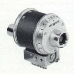
On the rear of the viewfinder is the parallax correction dial with the index mark on top. Rotate this dial in either direction until the distance from the camera to the subject is opposite the index mark. The illustration shows the parallax adjustment set at 10 feet. Either side of the double scale can be used.
