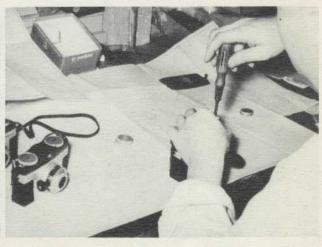
Assembler, Les Schwanbeck, tries to follow the blueprint while assembling knobs to the top of the otherwise completed A-4.
