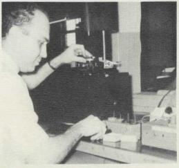
Jim Meldrum, Optical Engineer, checks the focal length of the shutter and lens assembly before inserting the proper shims.
