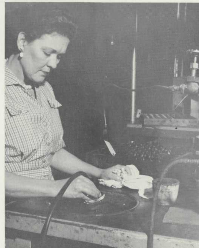
Edith Odegard uses a tub polisher to remove a water stain from a lens which will then meet Argus standards and be returned to production.
