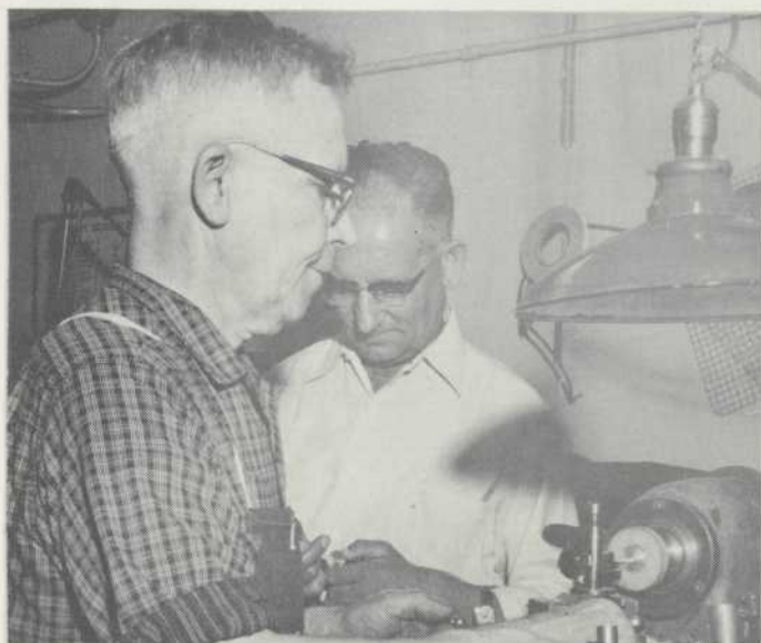
Delbert Cooper is reworking a part by diamond turning. Salvage Foreman Herman Bauer is checking dimension on a reworked part. Extreme accuracy is a keynote of all rework operations.
