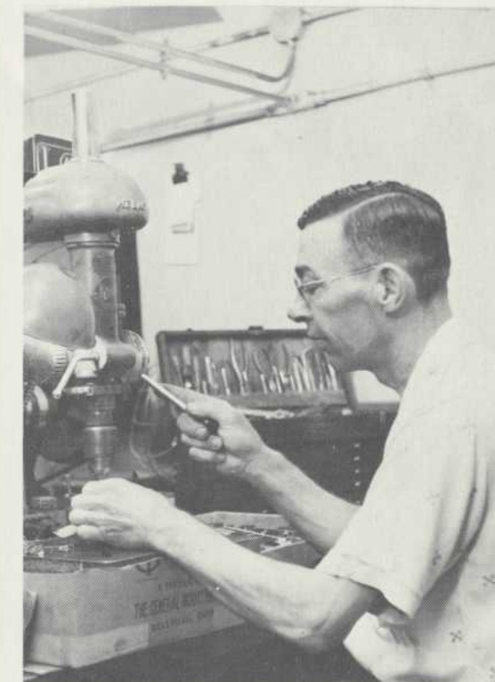
Harold Bailey in mechanical salvage is shown working at a drill press in a disassembly operation in preparation for reworking.
