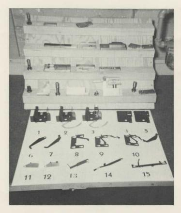
By designing these fixtures and die sets (upper portion of photo) for use with one air press, the Tool Engineering Department reduced the assembly area for producing these parts (lower portion of photo) to one station area, cut tooling costs in half, and eliminated operator fatigue and human error.
