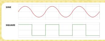
In synthesizers, sound waves are produced by electronic oscillators. These oscillators have a selector for waveforms and a control for pitch/frequency. The sound can also be changed in other ways via modulation.
