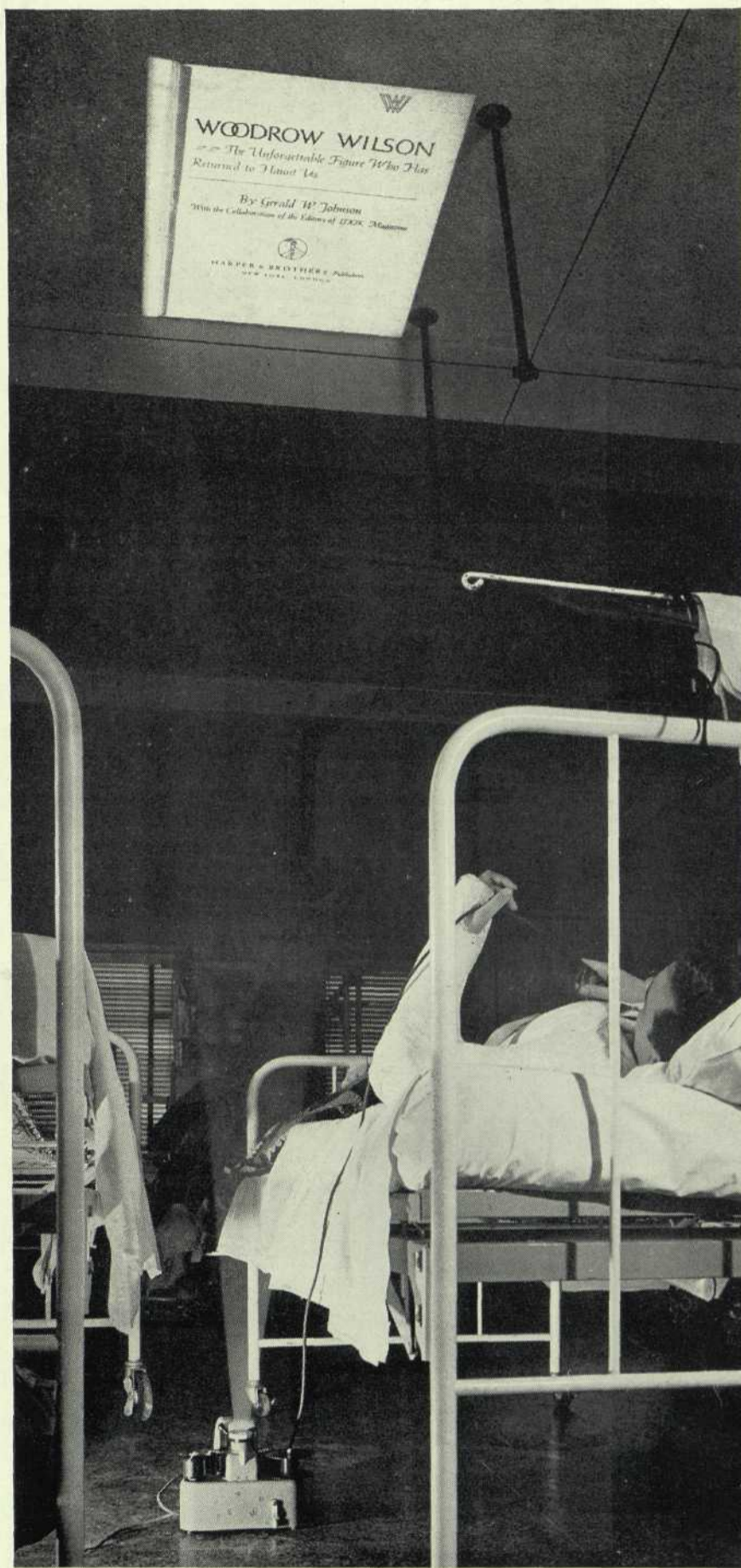
A clear, readable image is thrown onto ceiling directly over patient's head by small, 20-pound projector.
