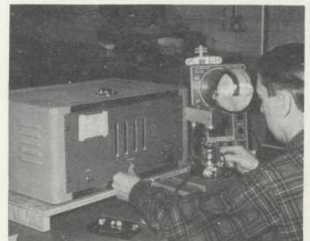
(Above) Eddie Girvan checks the shutter speed synchronization and electric circuits of the C-44.
