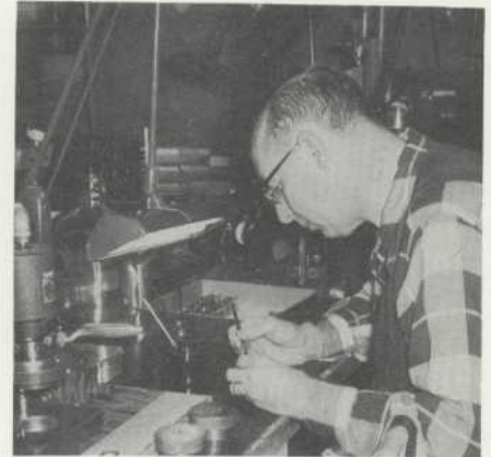
(Above) Ken Kaufman cleans a diaphragm assembly for the new four-element objective.
