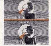
Turn the focusing ring until the split image in the clear center spot is aligned. (See illustrations at right.) You can also see the focus of the entire subject in the over-all viewfinder area surrounding the rangefinder spot. With the film wound, squeeze the shutter release slowly to take the picture. Use a tripod or other firm support for speeds slower than 1/30 second. To keep the camera steady when using slow speeds, operate the shutter with a cable release or by delayed action.
