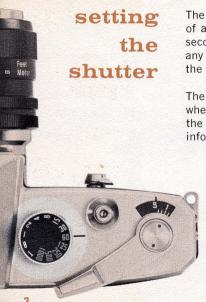
The numbers on the shutter speed dial represent fractions of a second—1 is 1 second, 2 is  $\frac{1}{2}$  second, 125 is  $\frac{1}{125}$  second, etc. The dial can be turned in either direction, at any time, to the desired speed. Be sure to set the dial on the detent of the number, not in-between numbers.
