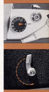
The size of the lens opening (f/stop or aperture) that will be set the instant you take the picture is determined by the position of the lens opening ring. Just turn the ring until the desired lens opening number is opposite the index mark. The ring can be set on the detents (click-stops) or between numbers. The correct lens opening to use for different films and lighting conditions can be found by using the Argus SLR Exposure Meter or by consulting the film instruction sheet.
