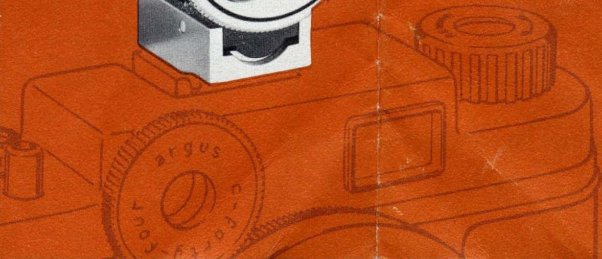
Your Argus Turret Viewfinder features a precision, selective optical system to show *exactly* what you are photographing with the 35mm Wide Angle, 50mm Normal, or 100mm Telephoto Lens. Your view will always be magnified to the full proportions of the viewfinder, *not* reduced in size. An efficient adjustment compensates for parallax—the difference which would otherwise occur between the views covered by the lens and the viewfinder. You see precisely what the lens sees—at all distances.
